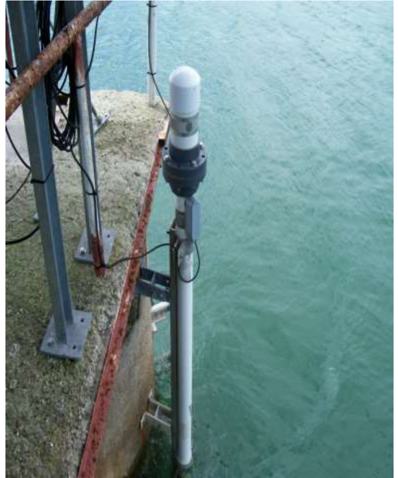
Four tidal gauge stations at Lamu, Mailindi, Kilifi and Shimoni for multi-hazard detection, ocean waves, sea level rise, salinity, sea surface temperature and water quality, including tsunami related at the Coast
