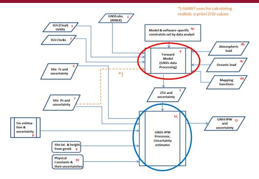
**Product traceability chain for GNSS-IPW** technique with standard GNSS data processing software and dedicated software package for IPW derivation and uncertainty estimation
