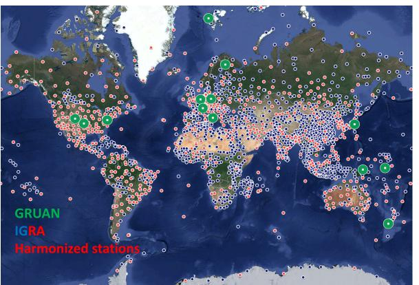
Global distribution of **GRUAN**Reference station (green large dots), **IGRA** baseline radiosounding stations (red and blue dots), and subset of IGRA stations harmonized using RHARM approach developed within C3S 311a Lot3 contract (red dots).
